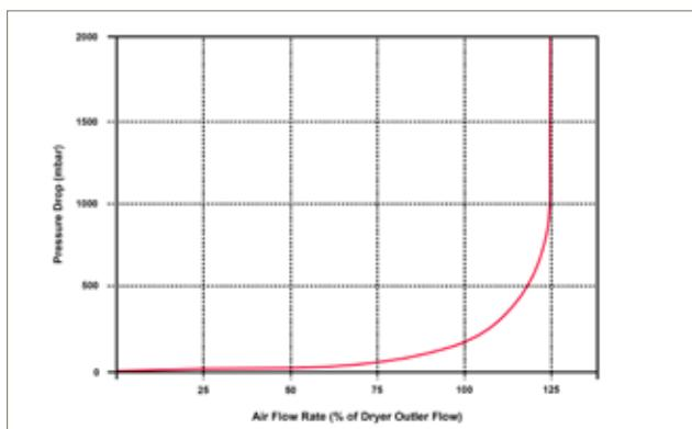
FCDs are installed in the outlet of a dryer and are sized so the maximum flow rate of the device is above the outlet flow rate of the dryer.
